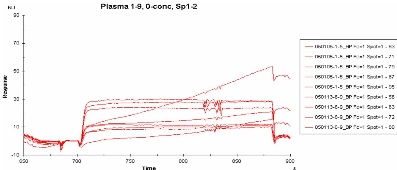
*Figure 23: An overlay-plot for blank samples (plasma 1-9) during the enhancement step. The sensorgrams have been obtained by subtracting the reference spot (spot 2) from the active spot (spot 1).*
