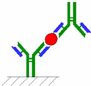
*Figure 8: Schematic picture of a sandwich assay. Showing the ligand (bottom), analyte (middle) and enhancer (top).*
