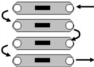
*Figure 3: The integrated microfluidic cartridge (IFC) in Biacore 3000. The IFC has four parallel detection spot over which a flow can be directed in either a serial or parallel manner. Here, a serial flow over the detection spots is shown. Figure from Biacore AB.*
