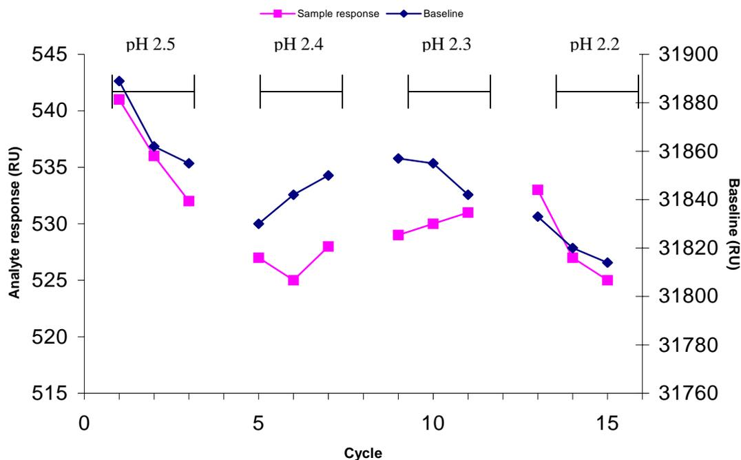
Figure 14: Result plots from regeneration studies on 1883 with four regeneration buffers with varying pH. The red plots correspond to analyte responses (left axis) and the blue plots are the values of the baseline response before the analyte injection in each run (right axis).
