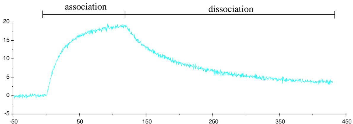
*Figure 4: Sensorgram showing the two phases of a reagent injection: association- and dissociation phase. Figure from Biacore AB*
