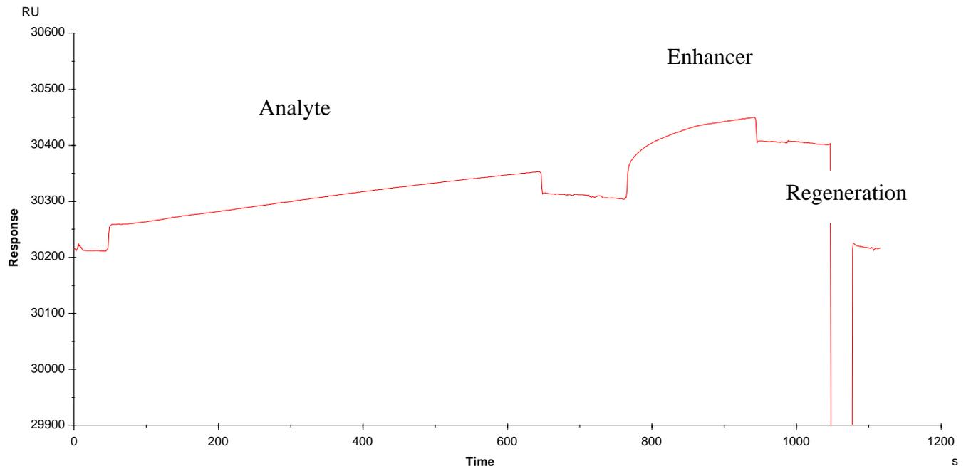
*Figure 12: Sensorgram showing an analysis cycle. The enhancer concentration is 35  $\mu\text{g/ml}$  and the analyte concentration 100  $\text{ng/ml}$ . The injection time was 10 minutes for the analyte injection and 3 minutes for the enhancer.*
