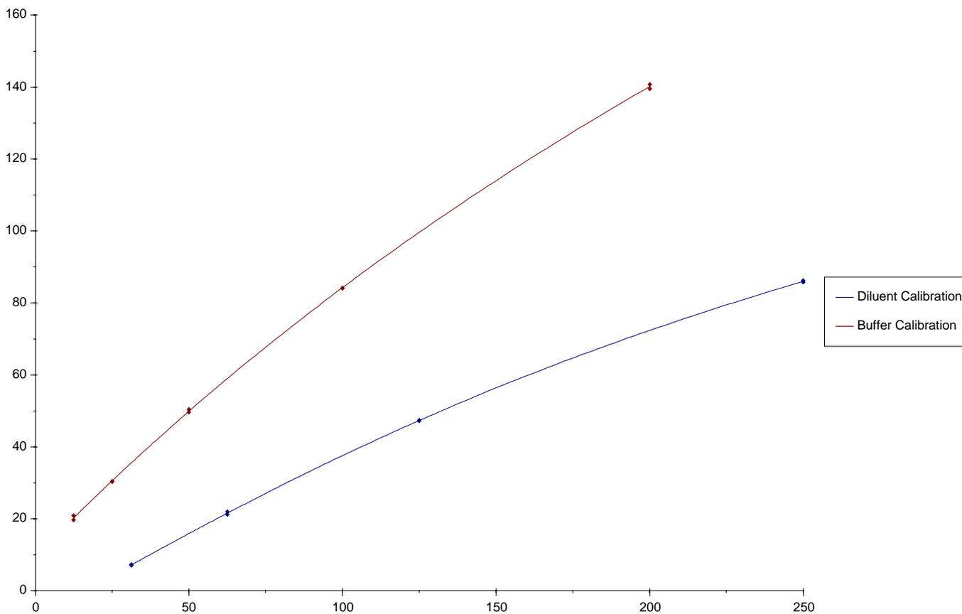
Figure 20: Calibration curves for PSA (250 - 30 ng/ml) in buffer (red) and diluent (blue).
