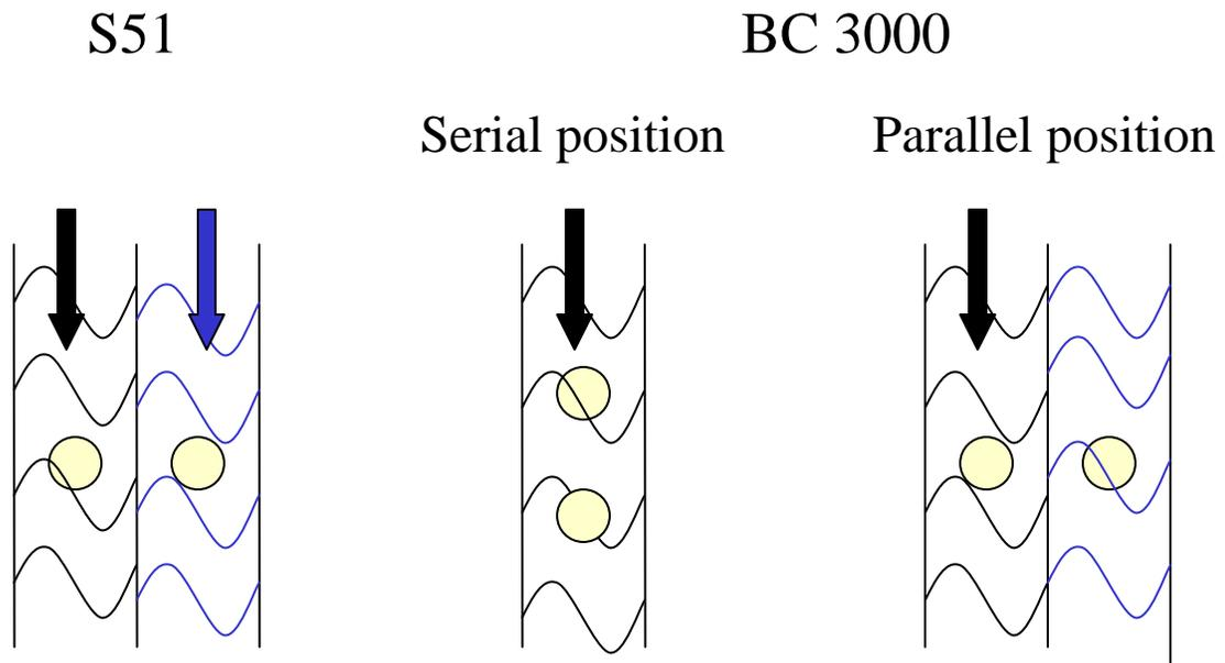
Figure 16: A schematic picture of the difference between the flow cells in S51 and BC 3000. In BC 3000 there are two ways for the detection, serial and parallel. An arrow symbolizes a flow of reagent; the black color symbolizes enhancement reagent and the blue running buffer.
