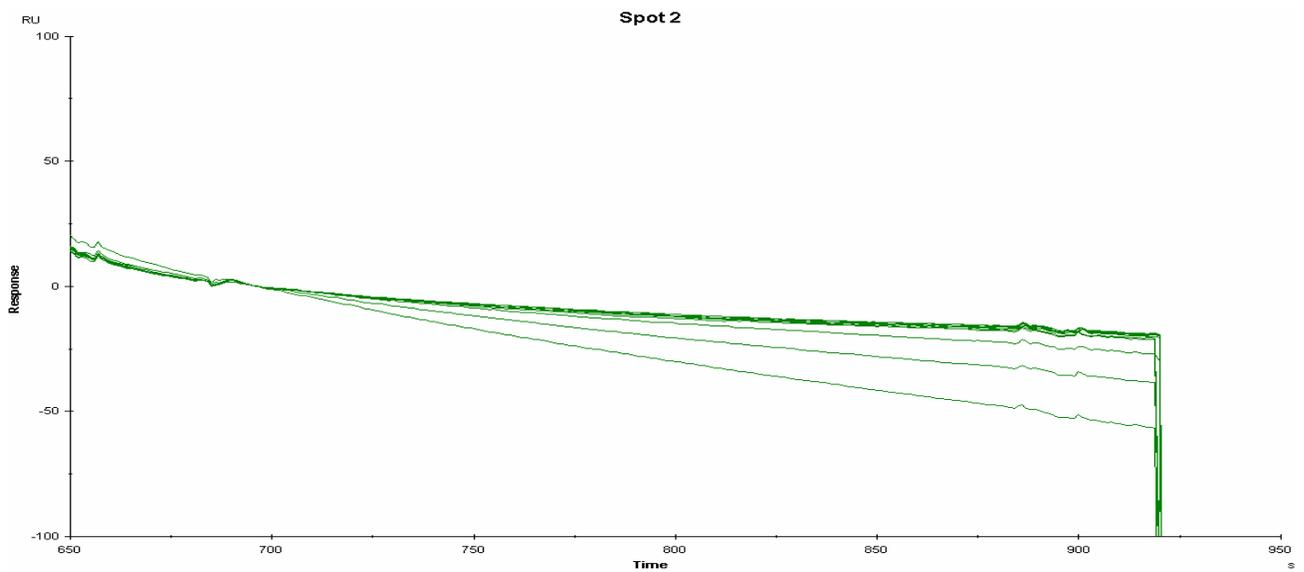
Figure 25: An overlay-plot for plasma 1 on the reference spot (spot 2) in a concentration range of 0-1000 ng/ml.
