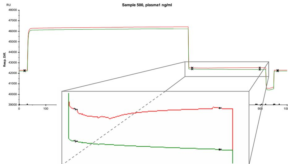
*Figure 9: A typical sensogram for measurement of PSA in plasma. The three phases of the assay can be seen: primary response, enhancement step and regeneration. The enhancement step has been enlarged in order to show the difference between the reference spot (green) and the spot over which enhancer is injected (red). Dissociation can be seen on the reference spot, while the enhancement injection can be seen on the other spot.*
