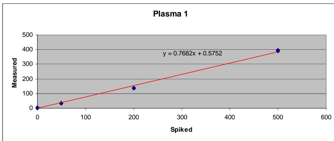
Figure 22: The spiked-concentrations plotted against the measured-concentrations for plasma 1, based on calibration curve in plasma 1. The level of recovery is 77 %.
