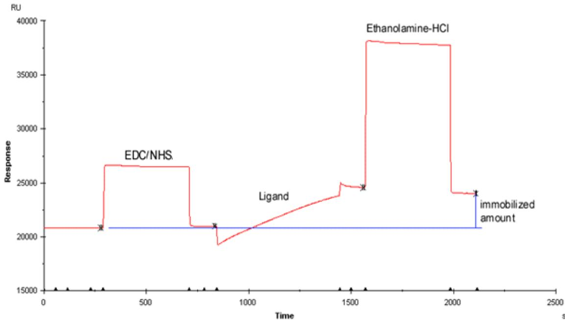
*Figure 7: A typical sensorgram where the ligand has been immobilized by amine coupling. The level of immobilized ligand corresponds to the difference in baseline level before and after injection of ligand. Figure from Biacore AB.*
