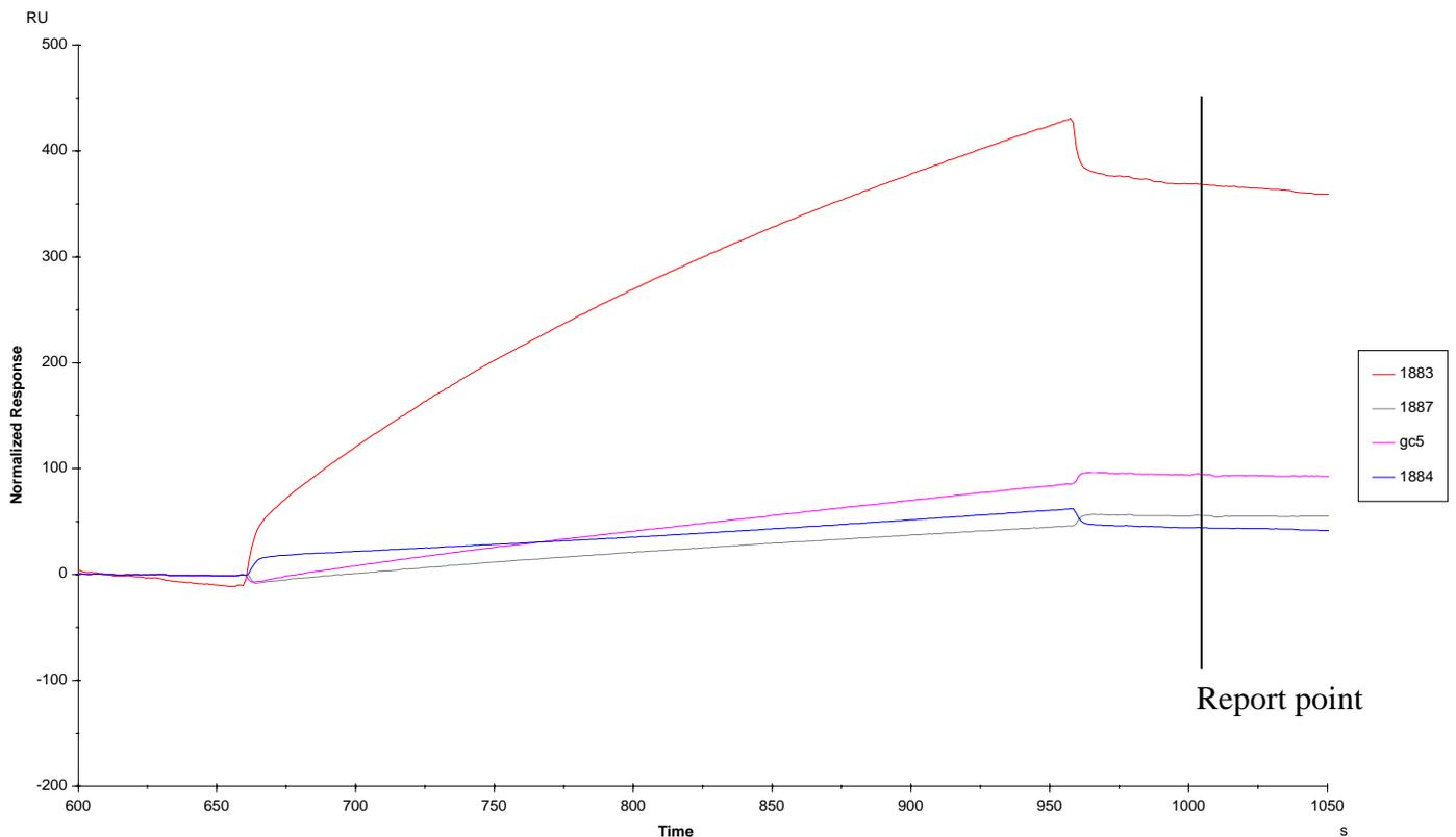
Figure 10: The over-lay plot shows the differences in binding levels between the ligands. Ligand concentrations were 30 µg/ml and the analyte concentration 1 µg/ml.
