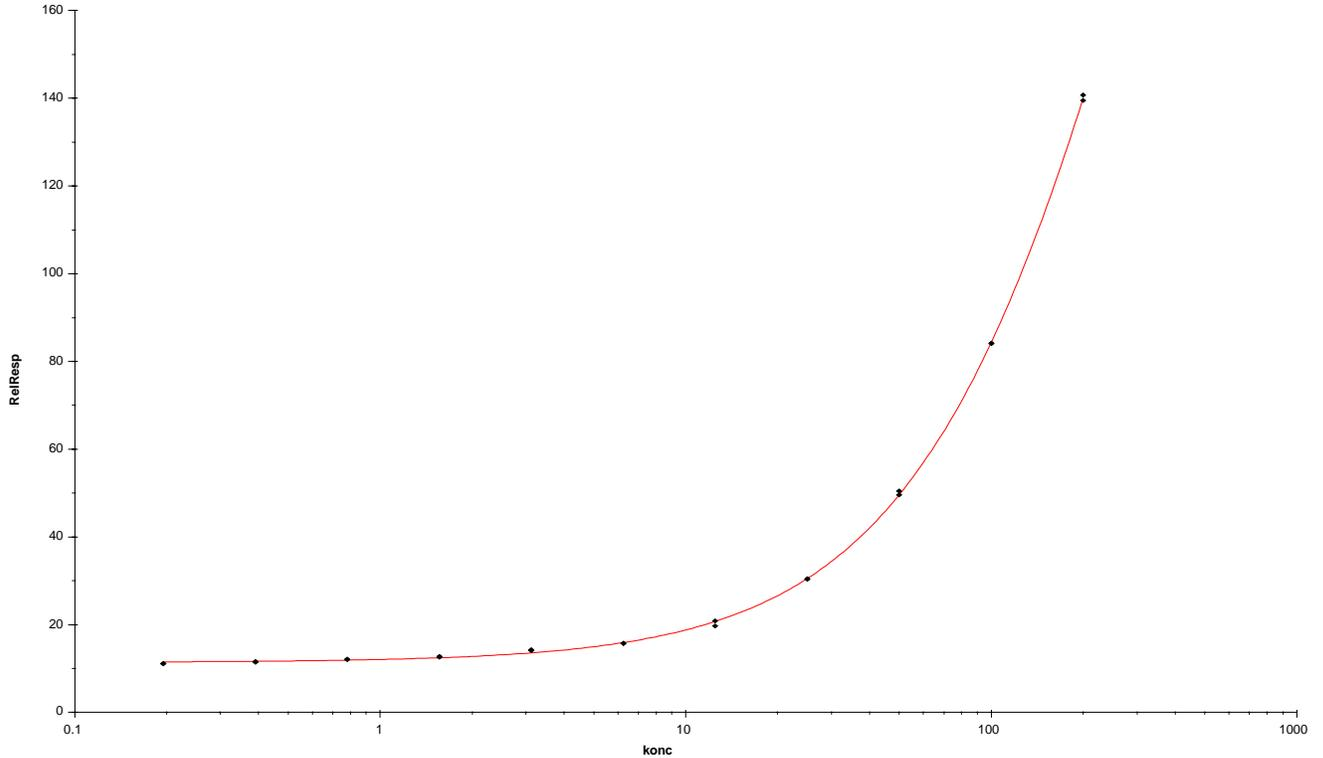
Figure 19: Calibration curve for PSA in buffer. The range of PSA is between 200 - 0.195 ng/ml. The curve was obtained by using corrected response values (spot 1- spot 2).
