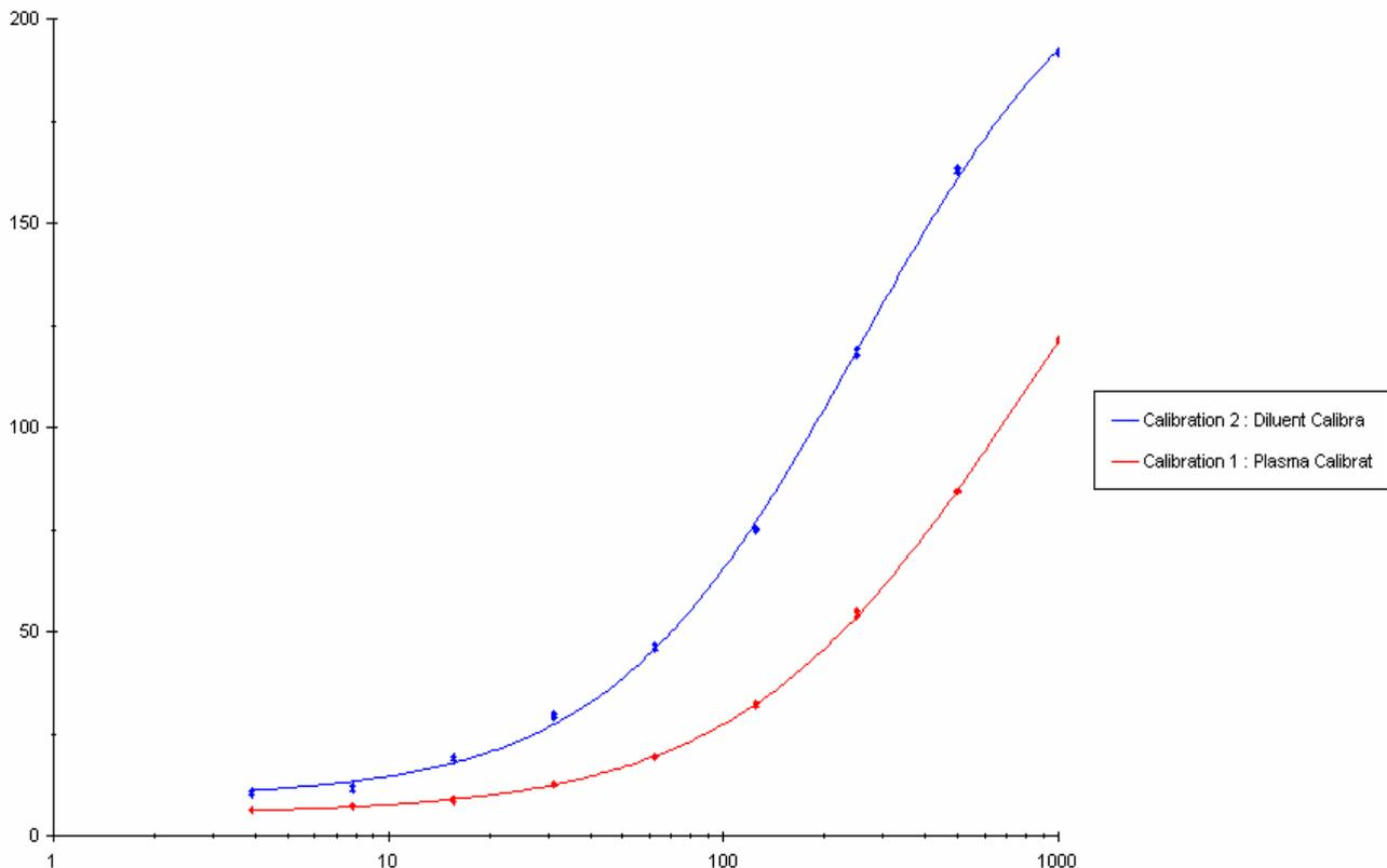
Figure 21: Calibration curve for PSA in plasma 1 (red) and HSA-solution (blue). The response (RU) is plotted as a function of concentration (ng/ml). The concentration range was 3.9 - 1000 ng/ml. The curve is obtained by using corrected response values (spot 1 - spot 2).
