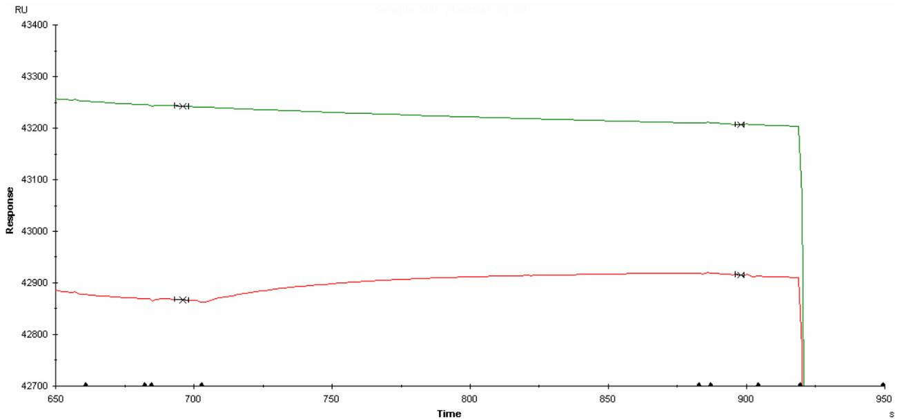
*Figure 18: Sensorgram showing the position of the report points: immediately before and after enhancement injection.*
