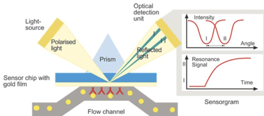
*Figure 1: The principle of SPR-detection. A mass change at the non-reflecting side (here illustrated with antibody-antigen binding), produces a shift in the SPR-angle. The shift causes a change in intensity, which is registered by the optical detection unit. Figure from Biacore AB.*
