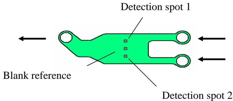
*Figure 2: The integrated microfluidic cartridge (IFC) in Biacore S51. The IFC has a Y-shaped structure and has two separate inflows for buffer/sample and one waste outflow. By controlling the flow rate during the coupling step, protein can be immobilized on one side or the other on the flow cell (spot 1 or 2). The middle spot cannot be used for ligand binding as is normally used as a reference spot. Figure from Biacore AB.*
