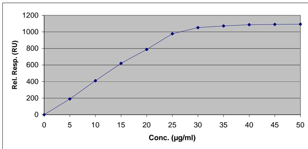
*Figure 11: Response as a function of enhancer concentration. The injection time was 3 minutes and the flow was 5  $\mu$ l/min.*
