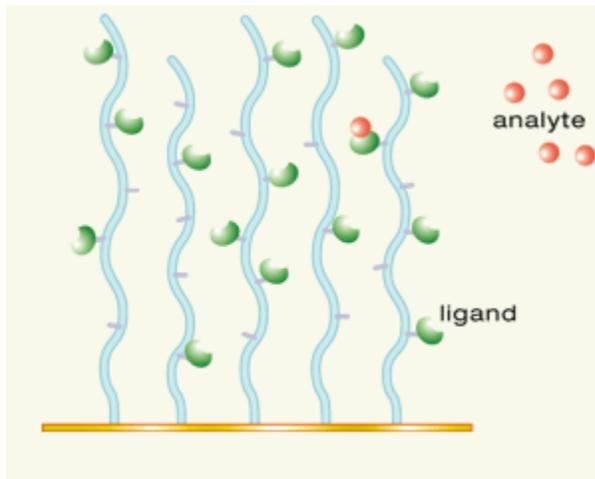
*Figure 5: Showing when an analyte comes loose from the ligand during regeneration. Figure from Biacore AB.*
