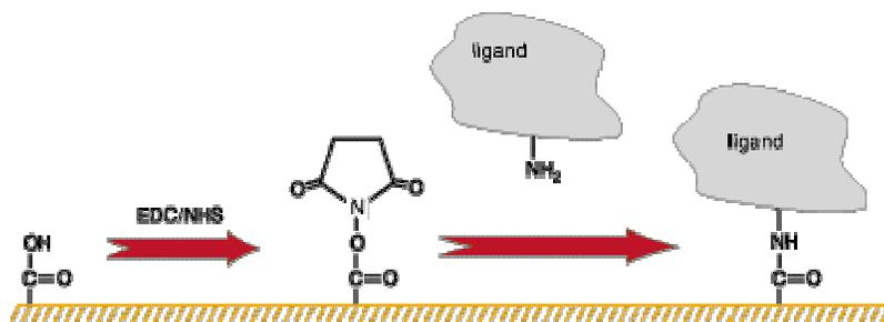
Figure 6: Scheme of amine coupling. Reactive esters are introduced to the surface by a mixture of EDC/NHS. The esters react with amines on the ligand and create a covalent link between the matrix and the ligand. Figure from Biacore AB.
