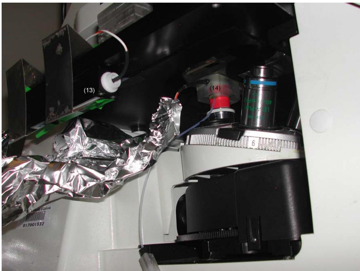
*Fig. 4. The lower electrode on the objective. See text for explanation.*
