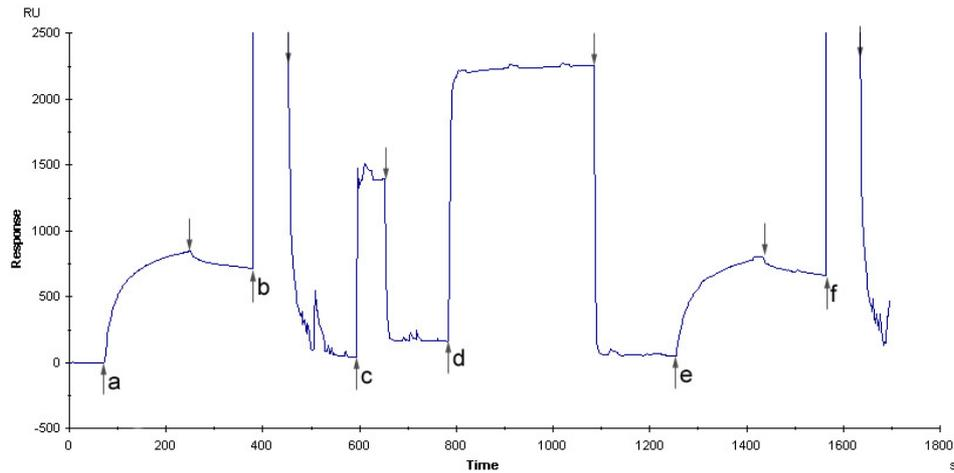
**Figure 10** Sensorgram from the 2000 RU-cell with the injections 2F9.1 ( $5 \mu\text{g ml}^{-1}$ , a),  $\text{MgCl}_2$  (4 M, b), OSR reagent (c), OG (30 mM diluted in HBS-N, d), 2F9.1 ( $5 \mu\text{g ml}^{-1}$ , e) and  $\text{MgCl}_2$  (f). Arrows indicate injection starts and ends.
