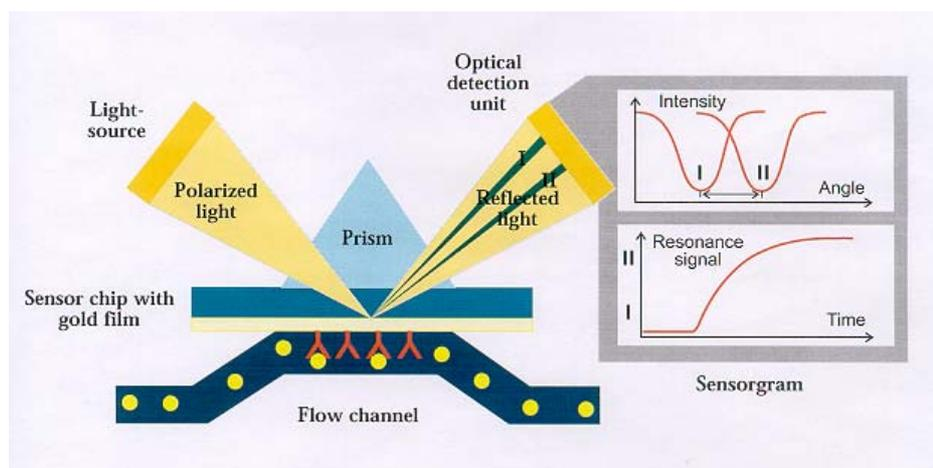
**Figure 1** Overview. Mass changes at the non-reflecting side (here illustrated with antibody-antigen binding) produce a shift in the SPR angle. The shift can be converted to a signal in a sensorgram. The illustration was used with permission from Anders Sjödin at Biacore AB.
