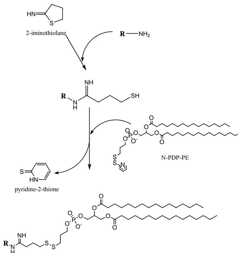
**Figure 8** Thiolation of antibody (**R**) followed by disulfide bonding of N-PDP-PE to the antibody. Upon the latter reaction, pyridine-2-thione is the leaving group.
