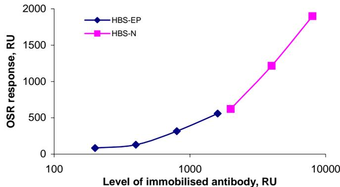
**Figure 21** Correlation between level of immobilised antibody and OSR response. Note that two different flow buffers have been used.
