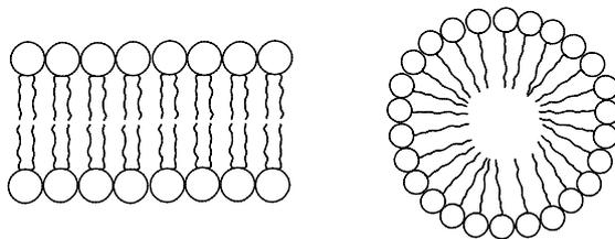
**Figure 5** Schematic pictures of a lipid bilayer and a micelle. The lipid bilayers can form large vesicles, liposomes, with diameters between 25 nm and 2.5  $\mu\text{m}$ .
