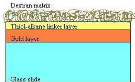
**Figure 2** Overview of a Biacore sensor chip. The ligands are linked to the dextran matrix.
