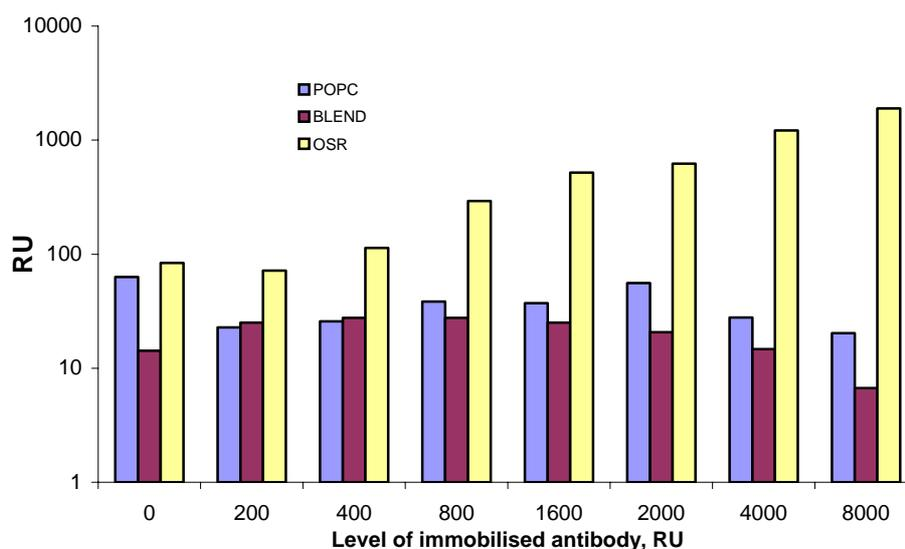
**Figure 22** Responses of the two different liposomes, POPC and BLEND, and the OSR reagent when injected over surfaces with conjugated antibody. Note the logarithmic scale on the y-axis.
