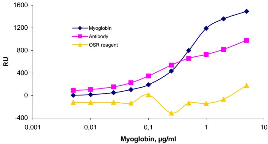
**Figure 19** Average values from a sandwich assay with varying concentrations of myoglobin. The myoglobin response is correlated to its concentration. So is the response for the conjugated antibody when the myoglobin concentration is less than  $0.25 \mu\text{g ml}^{-1}$ . The OSR response is not correlated to the antibody responses.
