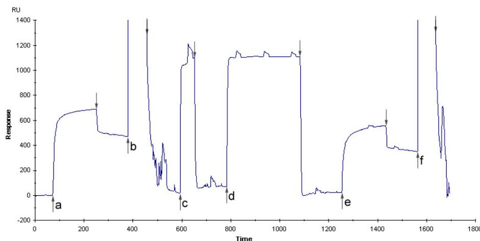
**Figure 9** Sensorgram from the 5000 RU-cell with the injections myoglobin ( $5 \mu g ml^{-1}$ , a),  $MgCl_2$  (4 M, b), OSR reagent (c), OG (30 mM diluted in HBS-N, d), myoglobin ( $5 \mu g ml^{-1}$ , e) and  $MgCl_2$  (f). Arrows indicate injection starts and ends.
