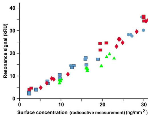
**Figure 3** Correlation between SPR and surface concentration for Chymotrypsinogen A (blue), anti-Transferrin (red) and Transferrin (green). The illustration was used with permission from Hans Sjöbom at Biacore AB.
