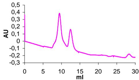
**Figure 18** Chromatogram from gel filtration of antibody conjugated with two molar equivalents of N-PDP-PE. The two peaks, corresponding to conjugated and non-conjugated antibody, are well separated and distinct.
