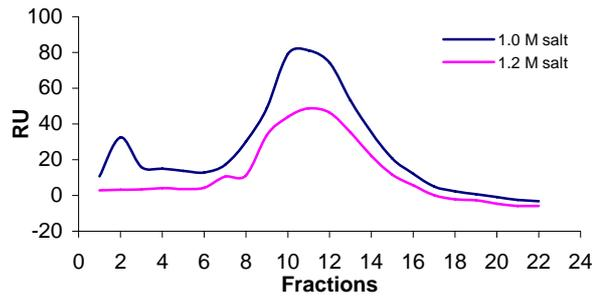
**Figure 12** Results from the Biacore tests of the fractions from the salt tests. The recovery of antibody is higher when a lower salt concentration is used.
