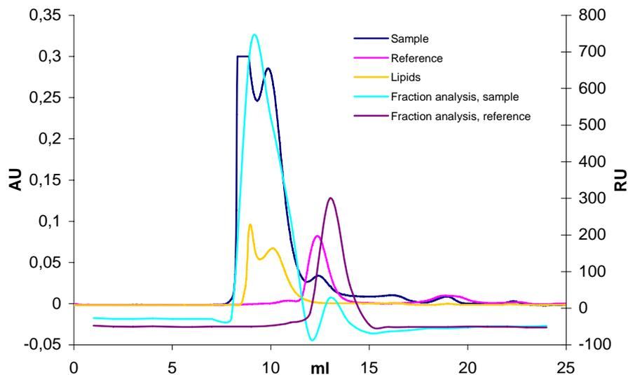
**Figure 16** Results from the gel filtration of conjugation with 100 times molar equivalents of N-PDP-PE. Note that the sample chromatogram was recorded on another scale than the reference and lipid. The figure also displays the results from the fraction analyses of sample and reference. Also note that the fraction analysis curves are slightly displaced compared to the chromatograms.
