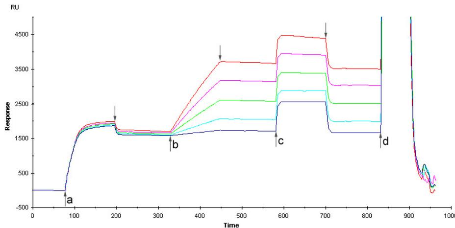
**Figure 11** Sensorgram from the sandwich assay. On a 2F9.1 surface, myoglobin ( $5 \mu\text{g ml}^{-1}$ , a), poly- $\alpha$ -myo (100, 75, 50, 25 and  $10 \mu\text{g ml}^{-1}$ , b) and OSR reagent (c) were injected. Arrows indicate injection starts and ends. The last injection is the regeneration with  $\text{MgCl}_2$  (4 M, d).
