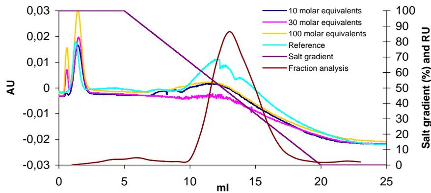
**Figure 15** Results from the HIC of the first N-PDP-PE coupling reaction, as well as the corresponding fraction analysis of the reference sample.
