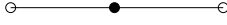
Figure 2: The figures illustrate the stencil used for the central differential approximations of first and second order in one dimension. The black grid-point is the one where the derivative is evaluated.
