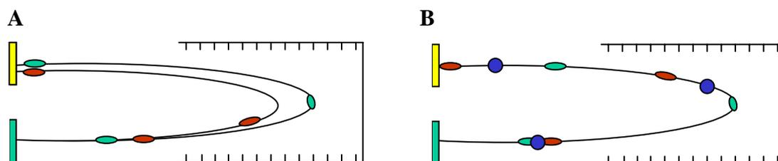
Figure 3. Two different ways in which the reflectron increases the resolution. A) Time-focusing; ions that have the same  $m/z$  ratio but different acceleration energies arrive at the detector at the same time because they are turned at different levels in the reflectron. B) The extended flight path increases the separation of ions having the same energy but different  $m/z$  ratios.
