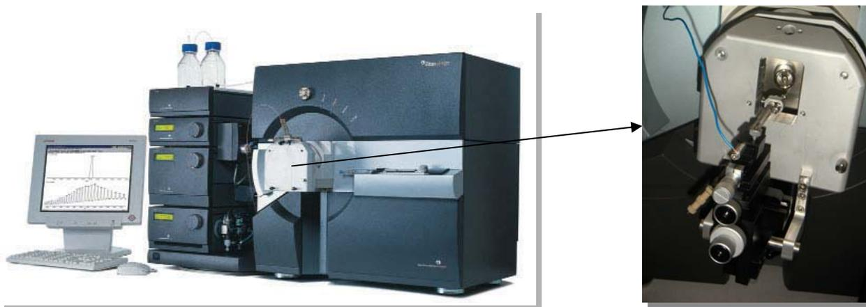
*Figure 13. The interface of the mass spectrometer was modified for nano-flow applications. A hole was drilled on the door to the interface and an x-y-z-table was mounted as above (right). A metal stick, on which the needle was attached, was placed on the x-y-z table so that the needle end could be placed just in front of the capillary entrance.*
