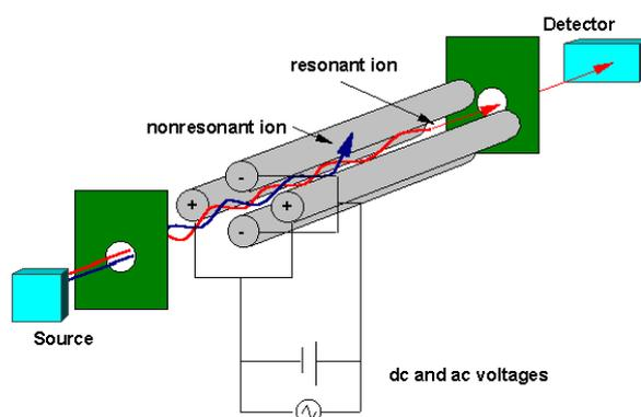
Figure 5. By applying the right *ac* and *dc* voltages, only certain ions are allowed to pass through the quadrupole and further into the collision cell. The ions of interest will resonate between the rods while the flight path of all other ions will be disrupted, as they collide with the rods. Illustration kindly provided by Marcus Svensson.
