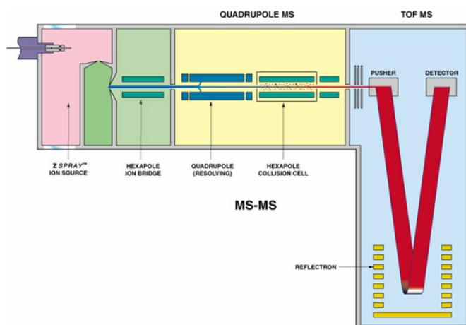
Figure 4. A schematic picture of the ESI Q-TOF mass spectrometer. This illustration was used with permission from Waters Corp.
