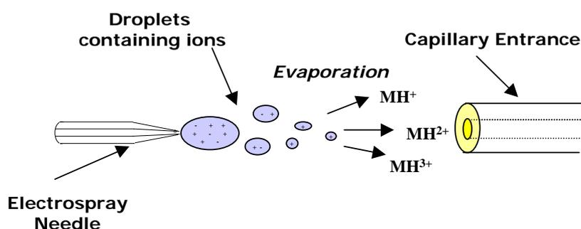
Figure 1. The principle for electrospray ionization.
