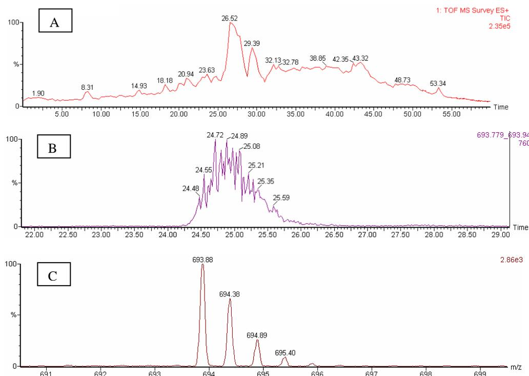
Figure 14. Examples of output data obtained from the mass spectrometer analysis. (A) represents the total ion current i.e. the sum of the intensities of all the peptide ions detected during the 60 min elution. (B) presents the EIC of the doubly-charged peptide ion with a  $m/z$  ratio of 693.88 Da displayed in the mass spectra in (C).
