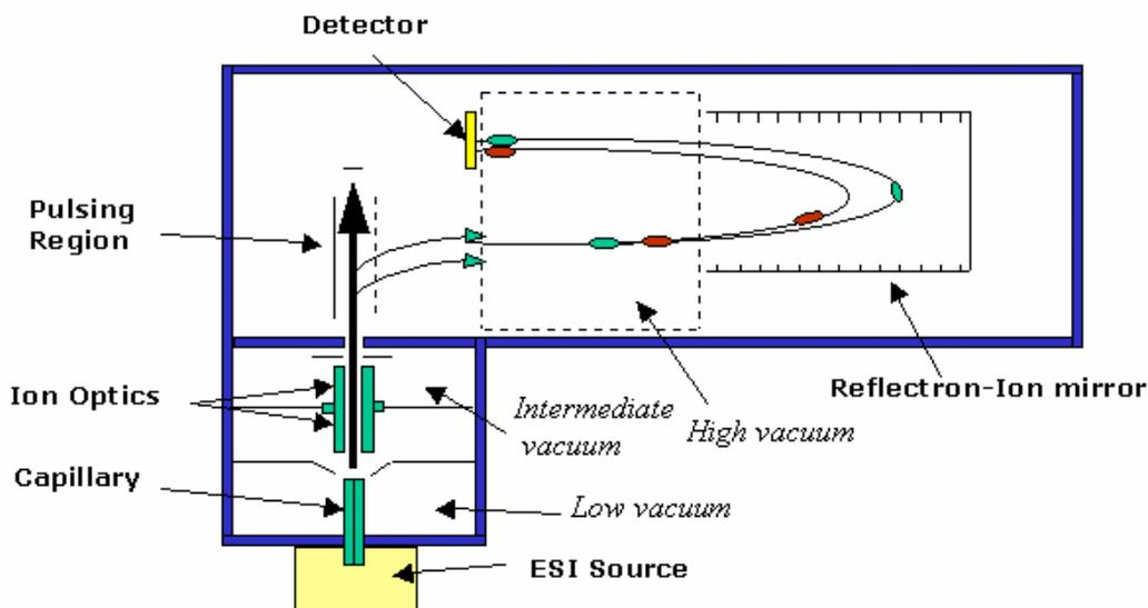
Figure 2. Schematic picture of the Ettan ESI-ToF mass spectrometer (Amersham Biosciences)
