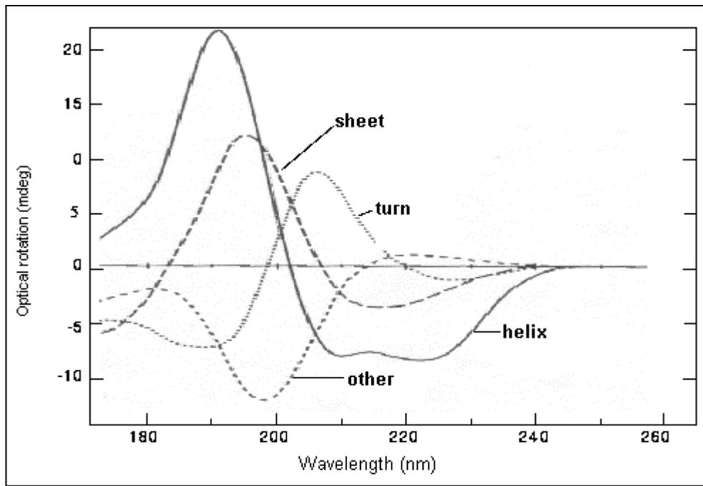
Figure 2.4: Circular Dichroism of different secondary structures.
