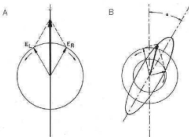
**Figure 2.3A: Linearly polarized light as a superposition of two rays that are circularly polarized in different directions. B: If absorbance and refractive index of a material is different for the two rays, it will cause ellipticity and optical rotation.**
