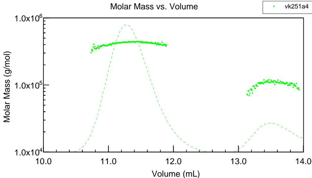
**Figure 3.4: Light scattering result from VCP K251A. The peaks are 90 degree light scatter and the dots correspond to the weight average molecular weight, which has been calculated from the light scattering.**
