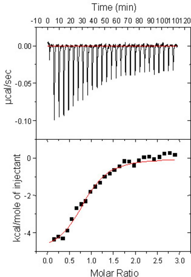
**Figure 3.14: Isothermal titration calorimetry of ADP added to VCP. Top: The differential power signal, i.e. the energy it takes to keep constant temperature in the reaction cell. Bottom: The integrated values ( $\Delta q_i$ ) per mole of added ADP.**
