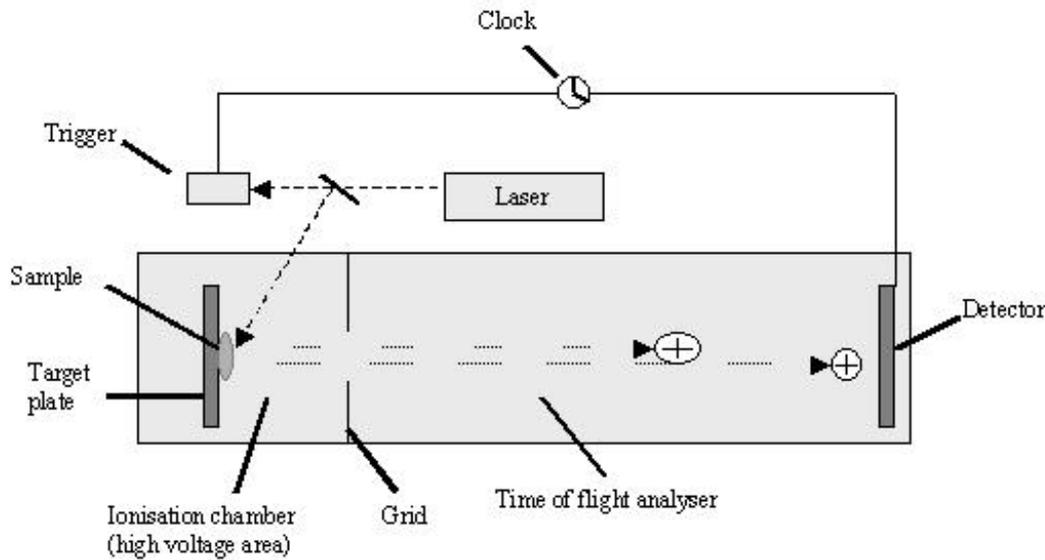
**Figure 5.** Schematic diagram of a MALDI TOF mass spectrometer.
