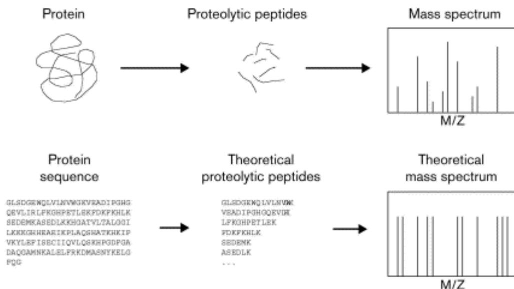
**Figure 6.** Protein identification using peptide mass fingerprinting [24]. The experimental mass spectrum is compared to theoretical mass spectra of a database.
