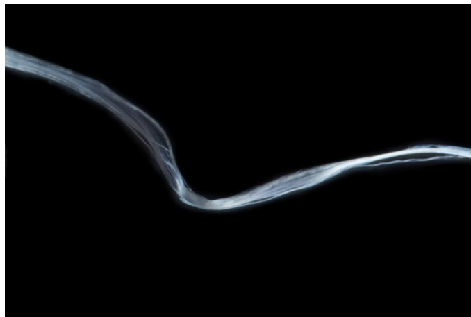
Figure: Fiber made of recombinant spider silk
